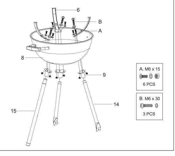
**Step 6:** Insert the bottom shelf(16) into the long leg(15) ends. the bent tip goes into the hole of the long leg first, then align and insert the other end into the wheel legs(14). then attach the air vent to the fire bowl(8) with the screws, washers and nut(A).
